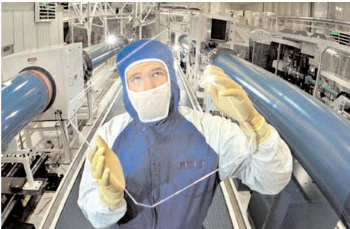
SURROUNDED BY Z-BEAMLET — Technologist Benjamin Thurston (1673) examines the debris shield that protects the giant Z-Beamlet laser's final focusing lens from flying debris when the Z accelerator fires. The lens is square because the beam generates an approximately 12-inch-square footprint, like a kind of flying pancake, until focused down to approximately 100 microns. (Photo by Randy Montoya)
