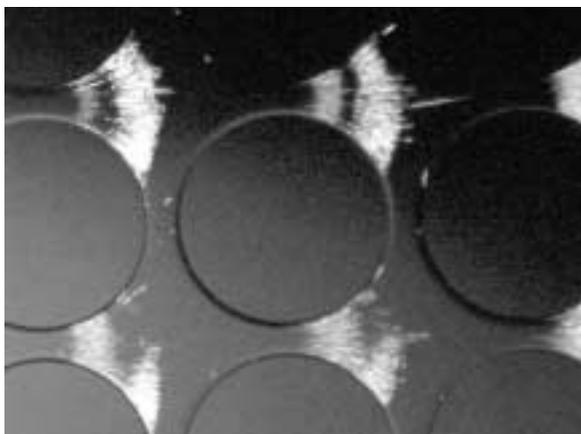
SEPARATING THE LIVING FROM THE DEAD — Across a microfabricated array of circular posts, dead and live *E. coli* bacteria collect into separate bands when a voltage is applied. Particles are repelled from the field between the posts because they are less conductive than the fluid. Live cells are even less conductive than dead ones, so are more strongly repelled and appear as outer bands. This phenomenon is being used by Blanca
