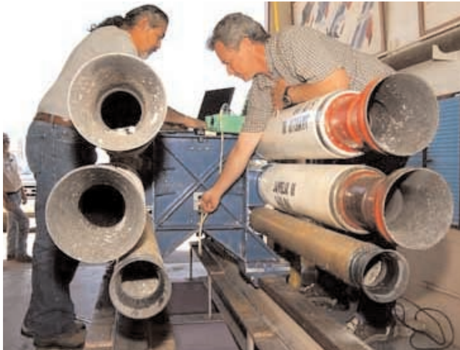
MONITORING ACCELERATION — Dave Faucett (2665, right) connects a data readout cable to an acceleration recorder while Phil Reyes (also 2665) uploads data following an April 30 experiment when a test unit was rocket-propelled along Sandia's rocket sled track into a water target. (Photo by Randy Montoya)
