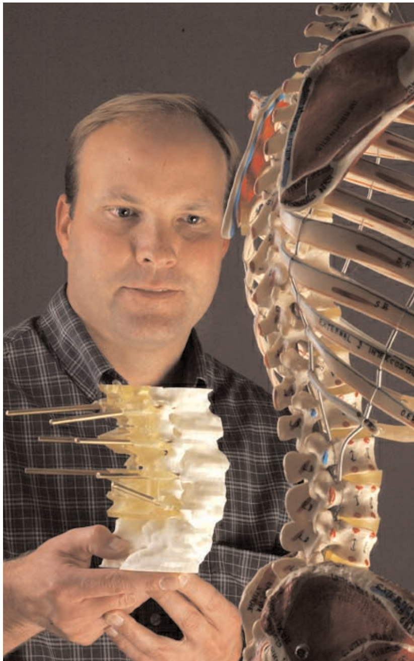
THIS IS SPINAL TAP — Terry Litts (14184) demonstrates a template developed using rapid prototyping technology. The template, which fits precisely over the target area of a patient's spine, allows an orthopedic surgeon to precisely control placement of the pedicle screws that are commonly used in spinal fusion surgery. (Photo by Randy Montoya)
