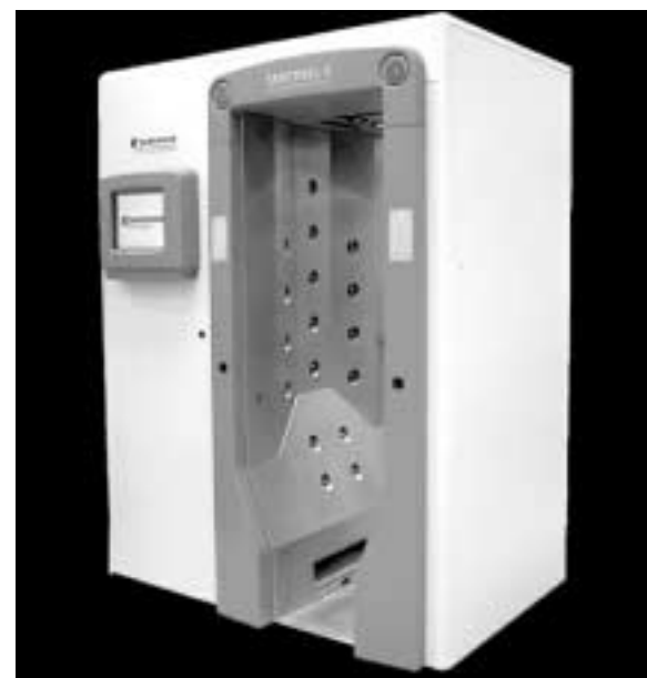
BARRINGER'S SENTINEL II walk-through portal can "sniff" seven passengers per minute for residues of explosives and other chemicals.
