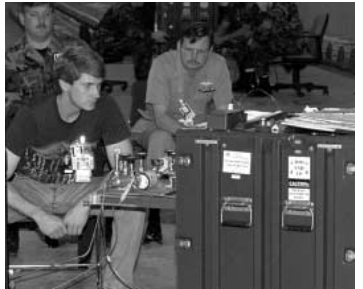
THE FIELD PORTABLE gas analyzer was designed, fabricated, and fielded to obtain internal dew point measurements on W80 warheads while in their stockpile locations. Here, Harry Cincotta (12332) performs a dew point measurement on a warhead using the device. This photo was taken in 1998 during a previous project involving the W80 warhead.
