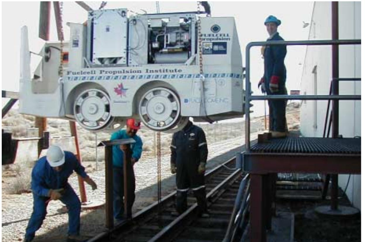
GETTING SETTLED — The crew positioned the mining locomotive, originally designed to run on batteries, on the sidetrack for test operation under hydrogen power. The test was conducted at Burlington Northern's yards in Reno, Nev.
