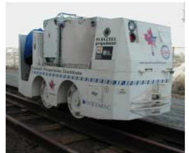
MOVING FORWARD — The mining locomotive ran on rails for the first time under hydrogen-fuel-cell power at a sidetrack in Reno.
