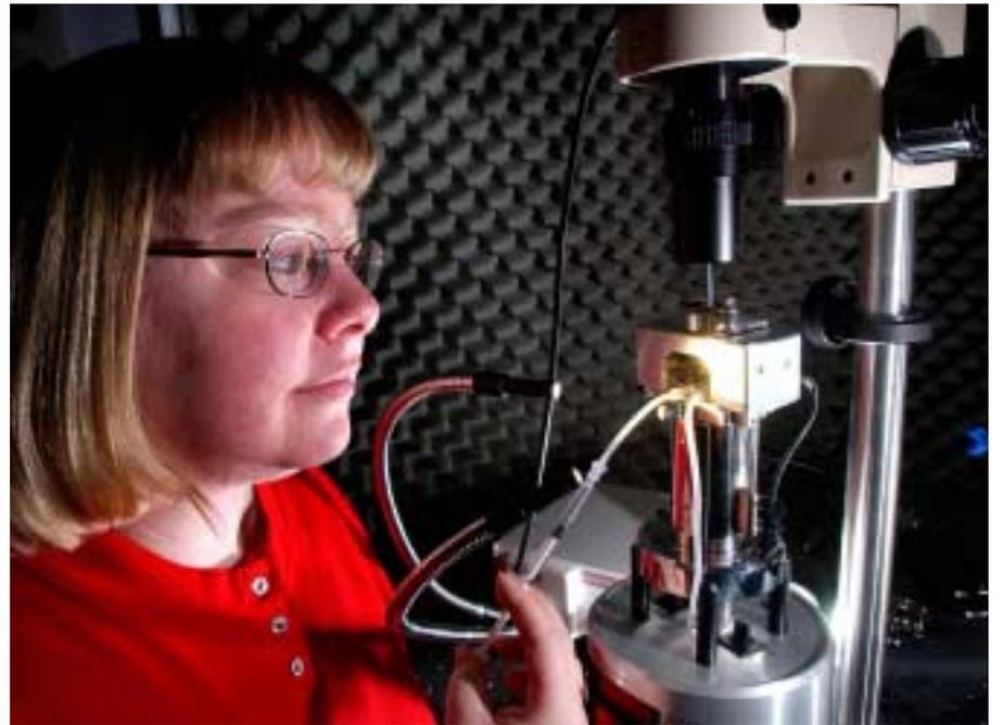
TRACKING RECEPTORS — Sandia postdoc Julie Last (1140) uses an atomic force microscope to image the travels of receptor-lipids on an artificial cell membrane. (Photo by Randy Montoya)
