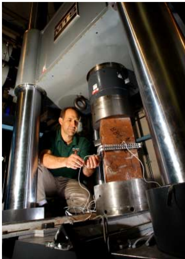
STRICT CALIBRATION — Dave Bronowski (6117) checks gauges on a 12-inch sample of tuff from Yucca Mountain. (Photo by Randy Montoya)
