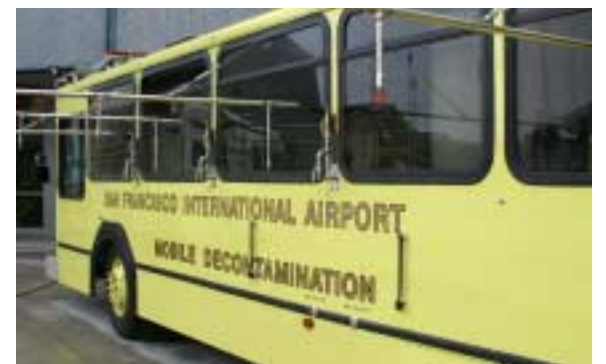
HAVE FOAM, WILL TRAVEL — The airport had a bus customized to administer decon foam and rinse off with warm water under shower heads mounted on each side.
