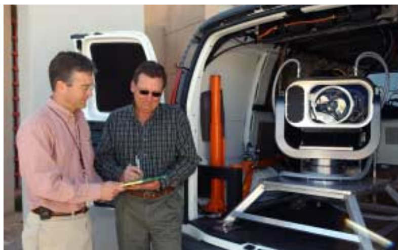
SKY SCANNER — Randy Schmitt (left) and Mark Johnson (both 1118) examine the Ares mobile biological weapons standoff detection system. (Photo by Randy Montoya)
