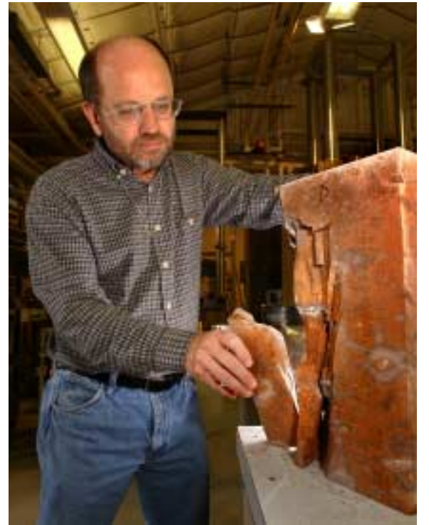
PIECING IT TOGETHER — Ron Price (6855) puts the pieces of this 12-inch tuff sample back together to better describe the failure mode. This sample cracked under about 600,000 pounds of force.
