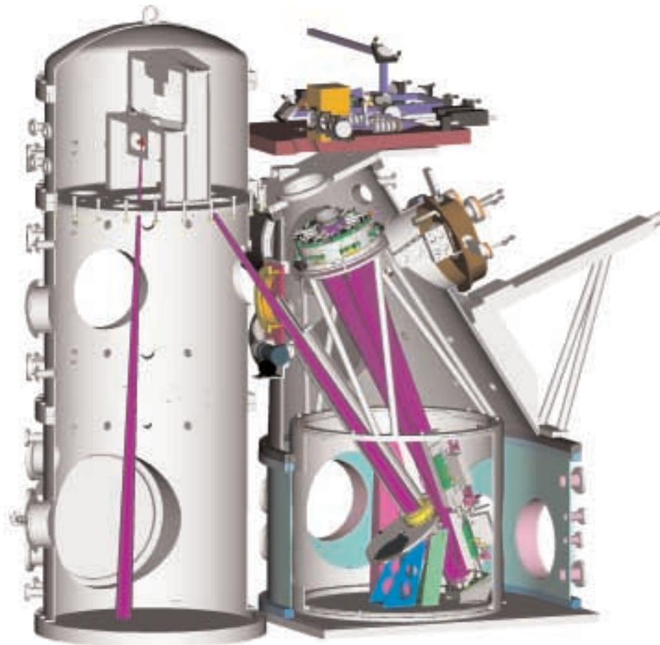
THIS COMPUTER-GENERATED illustration shows extreme ultraviolet light (EUVL) as a beam (shaded dark gray) being generated from a plasma source in the top right hand side of the apparatus, which was assembled at Sandia/California. The prototype machine was built by Sandia, Lawrence Livermore National Laboratory, and Lawrence Berkeley National Laboratory as part of a CRADA with a consortium of industry partners to support development of EUV lithography.
