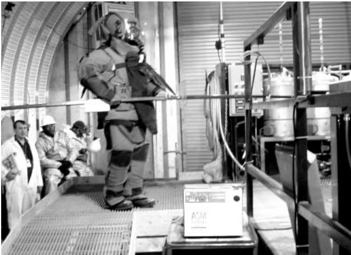
ARMY ORDNANCE EXPERT uses protective gear and a long pole to load the sarin-filled bomblets into the Explosive Destruction System at Rocky Mountain Arsenal.
