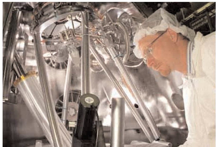
LINING UP — The Extreme Ultraviolet Lithography tool, shown here being aligned during its assembly at Sandia/California, is now subject to industry interactions in a Resource Development Center. Through tests conducted at this user facility, tool-making manufacturers are developing new commercial chip-patterning devices to supply the microchip manufacturing industry. (Photo by Randy Montoya)
