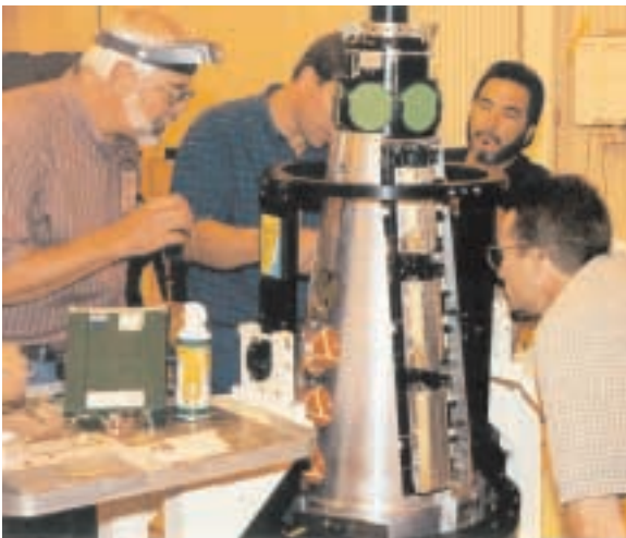
PREPARING AN RV-like platform called a target deployment structure (TDS) prior to the RCT-2 test were (left to right) Mel Krein (15415), Brian Pardo, Jim Aldaz (both 15413), and Rob Brown (15414). Target objects that look like pucks (top of TDS), balls (left side of TDS), and cannisterized balloons (right side of TDS) are visible.
