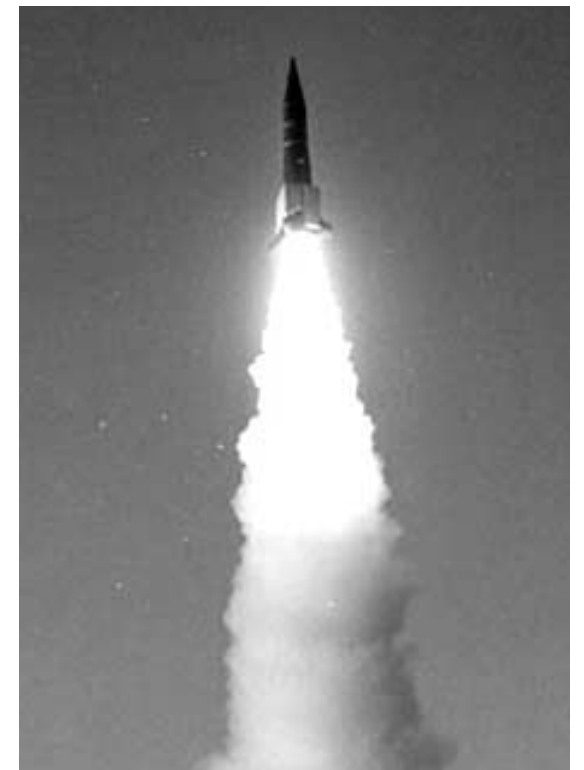
TARGET VEHICLE (based on a modified Minuteman I second stage rocket motor) lifts off from the Kauai Test Facility Jan. 25. (Photo by Diana Helgesen, 15419)
