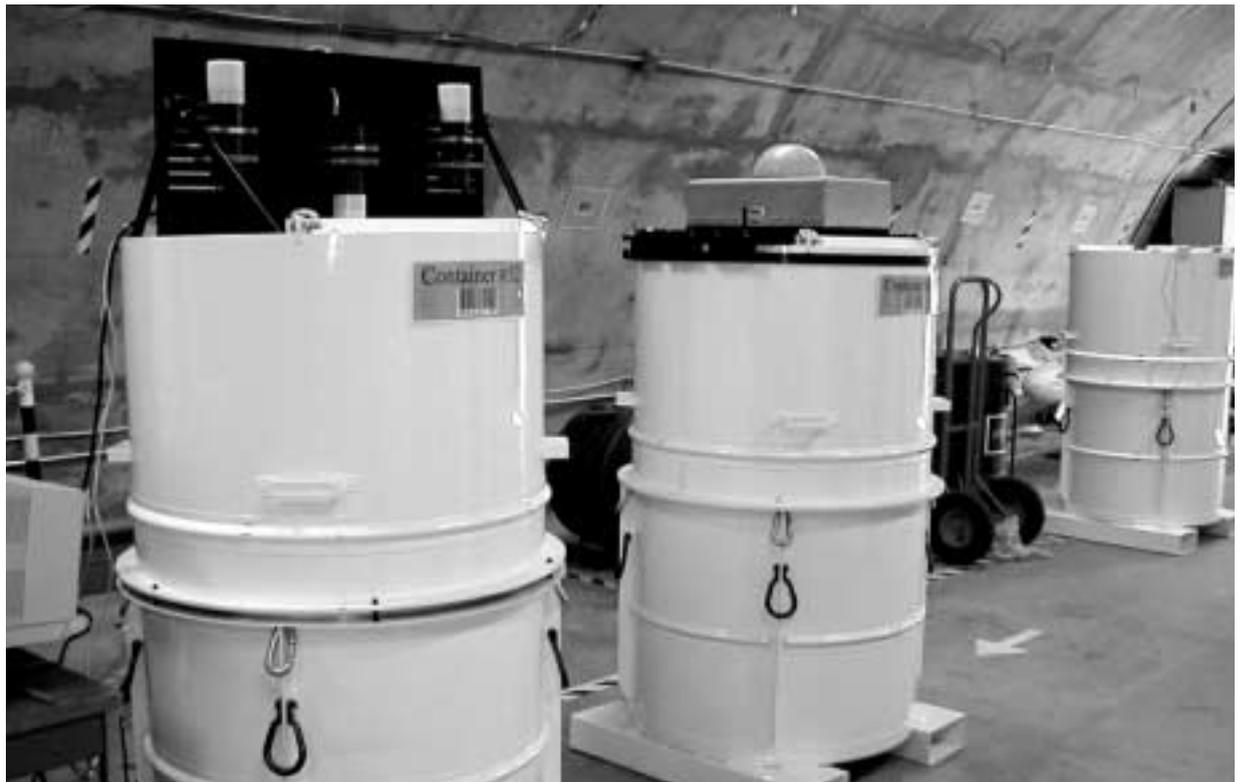
THE MOST RECENT version of the Radiation Continuity Checker is shown at left, atop mock warhead container #52 in a bunker at Sandia/New Mexico. This version uses active collimation to eliminate background radiation, which obviates the need for heavy shielding around the detector.
