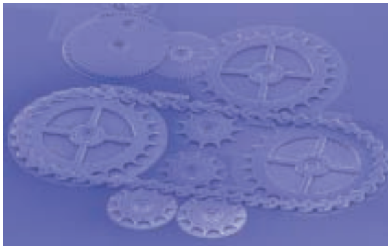
OVERVIEW — Pictured is a microchain. The distance between chain link centers is 50 microns.
