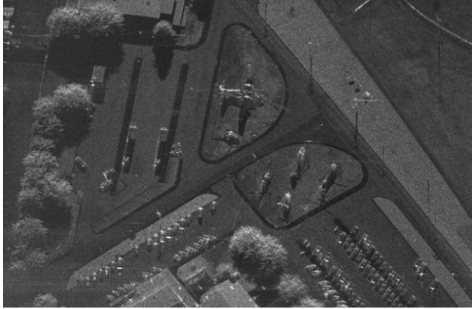
Figure 6. SAR image with illumination corrected.
