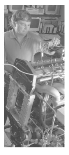
Pete Witze operates a specially instrumented engine that allows optical studies of fuel injection at the Combustion Research Facility in Livermore, California.
