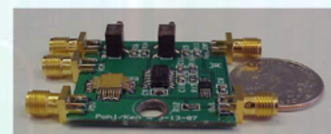
Packaged Accelerometer and PCB Readout Electronics
