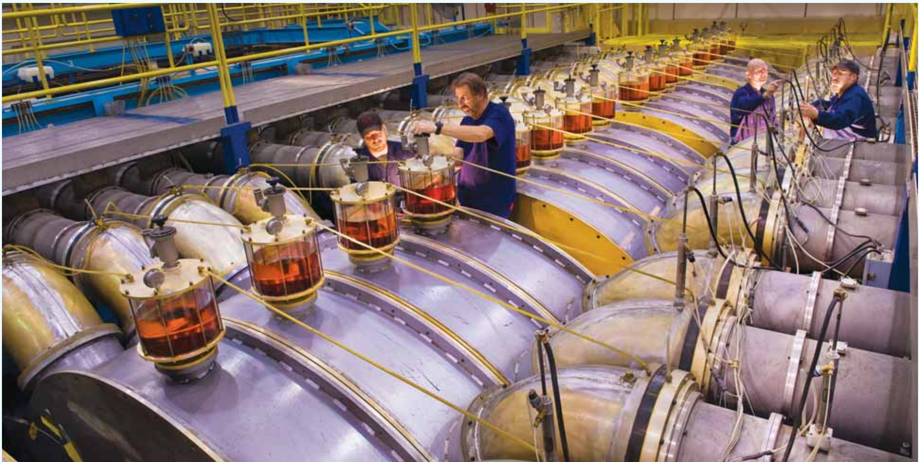
THE LINEAR HERMES pulsed power machine — the most powerful gamma ray producer in the world — is serviced for its next shot by technicians, left to right Chris Kirtley, Gary Tilley, Harold Brown, and Jose Montoya (all with Raytheon K-Tech). Because of Sandia’s nuclear responsibilities, Hermes and Saturn are kept in “warm, standby mode” for immediate testing of components.
