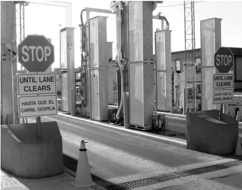
THE NEW YORK CONTAINER TERMINAL site configuration included several Advanced Spectral Portal primary stations, one of which is shown here.
