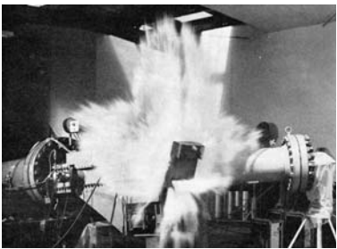
WATER BURSTS from the muzzle of the "squirt gun" as the steel door is released.
