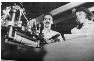
DANGEROUS JOB — An instrumentation package developed by Sandia enables this robot to develop a 3-D map of a simulated underground waste repository.
