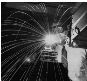
A spray of molten droplets produced when spinning rod of alumina ceramic is melted by infrared energy from a carbon dioxide laser.
