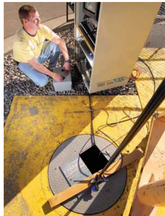
A DEFT TOUCH — Don Hanson (1382) controls the movements of Swarmy the robot in an old wastewater storage tank 26 feet underground, an environment not safe for human entry. (Photo by Randy Montoya)
