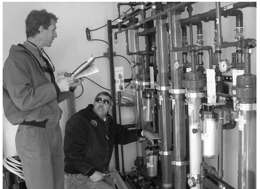
BRIAN DWYER and Randy Everett, both 6118, check out equipment to be used in experimental methods of treating arsenic-contaminated water.
